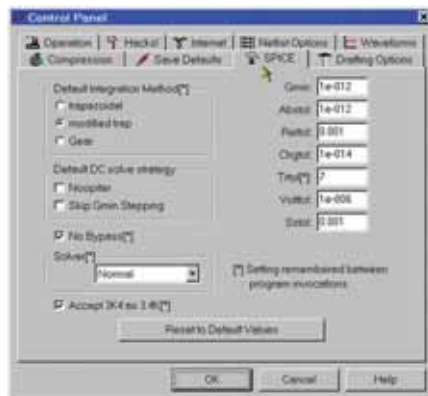
Obr. 2 – Nastavenie programu cez Control Panel.tif
